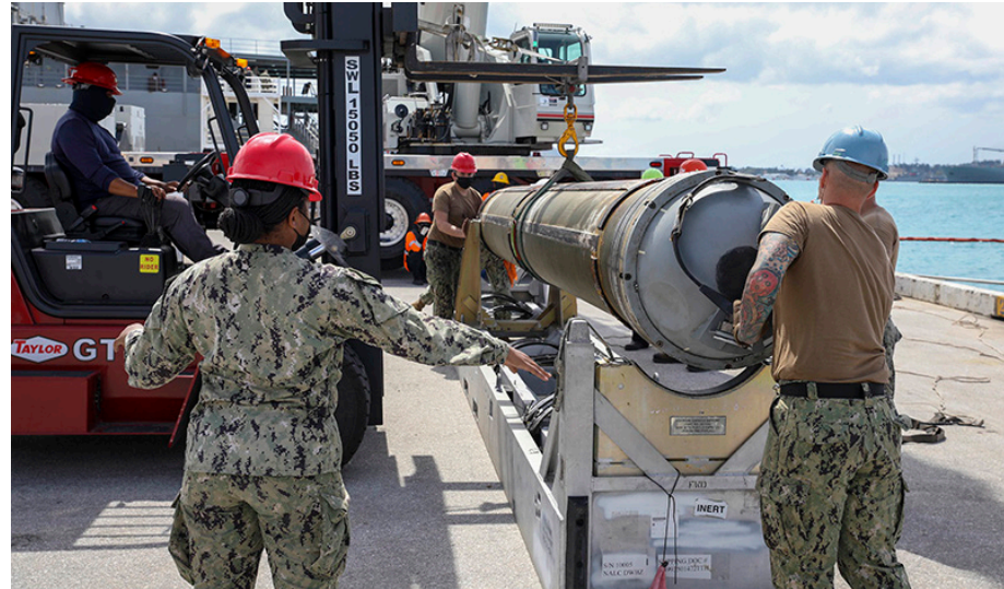
Sailors assigned to the submarine tender USS Emory S. Land (AS 39) weapons handling division conduct an offload of a Tomahawk missile from the Los Angeles-class fast-attack submarine USS Asheville (SSN 758), February 1, 2022.
